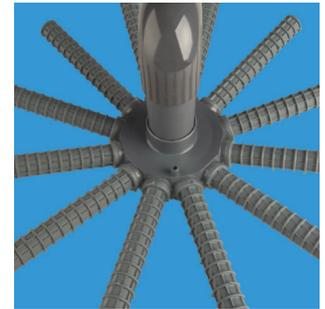
The Aster Series filter utilizes 1" laterals made from injected molded polypropylene. Each lateral is slotted 360 degrees to provide superior filtration and a quick complete backwash cycle.
