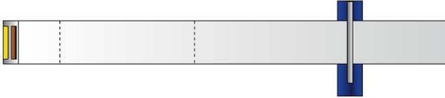
2. Slide the heat shrink on the strip light. Then slide the plastic retainer on. Make sure the ribbed side faces the non-LED side.
