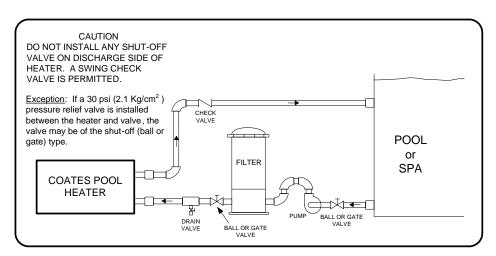
FIGURE 1 - PIPING DIAGRAM
