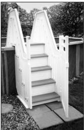
Assemble both units and position the in-pool unit in the desired location, after filling it in the same manner as step #12. Allow approximately two (2) inches of clearance between the side of the pool (pool liner) and the Entry System. Make any necessary height adjustments to ensure that all four (4) threaded adjusters are supporting the unit, that the unit is level and does not wobble, and that the underside of the top step is about (1/2) inch above
