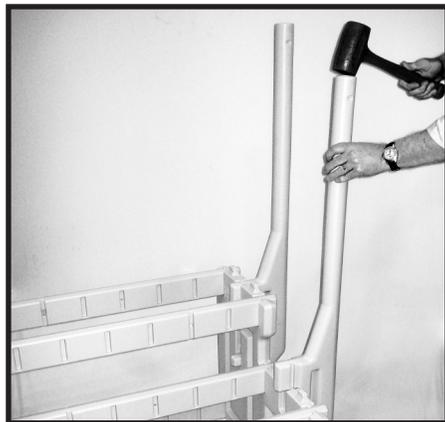
**Step 4:** Using a rubber mallet, install the four handrail posts into the middle slots of the top two step locations on the left sidewall, and the top two step locations of the right sidewall. Handrail posts must be seated into the slots.
