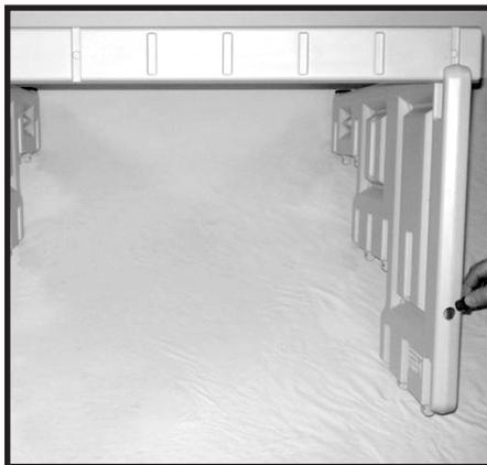
**Step 2:** Using a rubber mallet install one of the 3" supports into the slot located on the bottom of sidewall. [36" step will have 2 sidewall, 74" will have 4 sidewall]. Install one plug into each sidewall.
