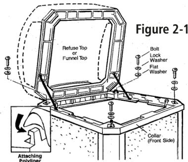
4. Starting with the hinged side of the collar (see Figure 2-1), use flat head screwdriver to loosen (2) bolts, (2) lock washers and (2) flat washers. Place bolts and washers to the side.
