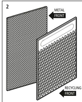
2. Identify the front of the (4) decorative panels. For recycling panels, the waste stream label should face outward. For metal decorative panels, the flat face should face outward.
