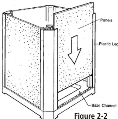
8. Press panels firmly into the channels in the base until they are securely seated.
