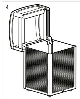
4. Press panel firmly into the channels in the base until it is securely seated.
