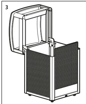
3. Slide (1) panel into the channels in the metal legs, in front of the metal backplate, with the facade facing out. Do not drop into place.
