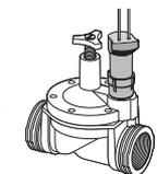
**NOTE:** For all brand name valves with internal manual bleed lever, make sure the lever is in closed position. Do not move the lever after installing the solenoid with the valve adapter. If the manual lever on the valve is used, it can damage the adapter or the sleeve causing the valve to stay open.
