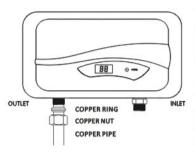
This water heater is supplied with 1/2" compression fittings, Do not weld or use Teflon or paste.
