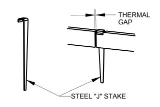
3c USE A STEEL HAIRPIN LEAVING A GAP FOR THERMAL EXPANSION
