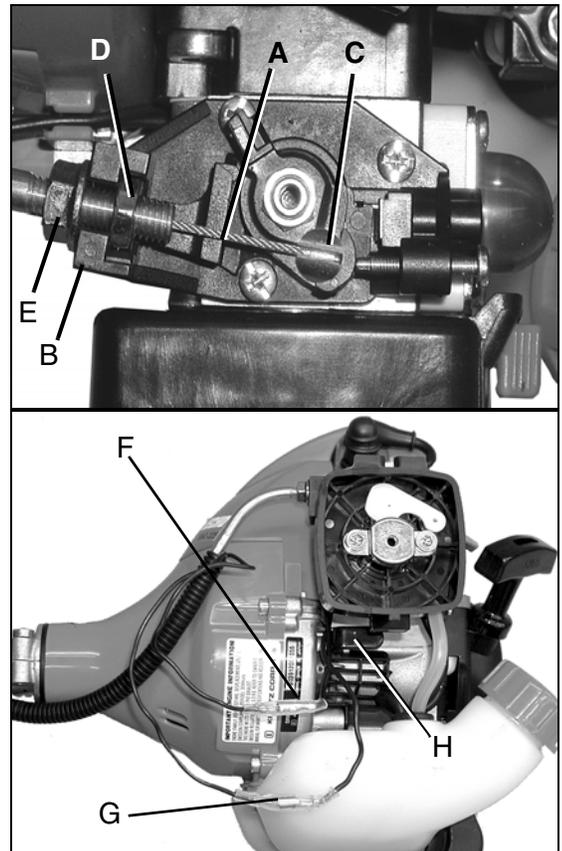
5. Secure ignition leads against engine housing with clips (H, I).
