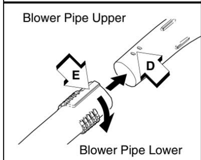
Note: Blower use will eventually loosen pipe connections. Exclusive positive locking system allows pipes to be tightened. If loosening occurs, remove lower straight pipe, and install according to instructions 3 & 4.
