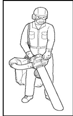
Note: Vacuum action works best at higher engine speeds. Avoid using vacuum in areas where rocks or other large, hard debris may be vacuumed into unit. Clear these areas with blower first, blowing light debris into a pile. Use attachment to vacuum pile.
