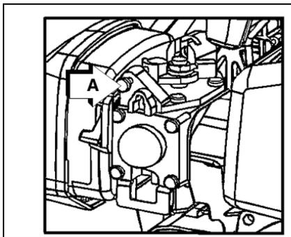
3. Check idle speed and reset if necessary. If a tachometer is available, idle speed screw (A) should be set to the specifications found on “Specifications” Page of this manual. Turn idle screw (A) clockwise to increase idle speed; counter clockwise to decrease idle speed.
