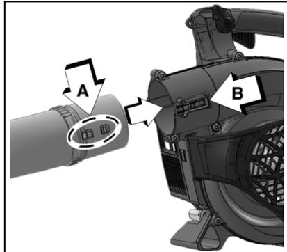
Do not assemble the opposite end of the upper blower pipe to the fan case.
