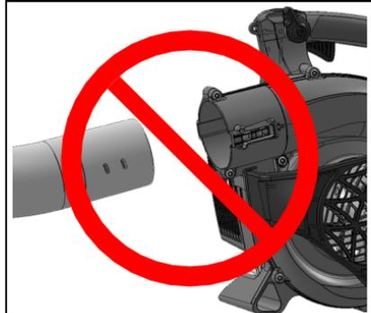
3. Align tabs (C) with grooves (D) and slide lower blower pipe (E) over upper pipe (F) until there is light resistance. Do not force the connection.
