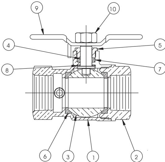
1. Body - Lead Free\* Cast Copper Silicon Alloy
