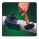
Apply wedge half way by hand and finish off with a slight tap of a rubber mallet.
