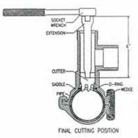
Using a socket wrench with a 6" extension, turn the cutter clockwise to cut an opening in the pipe. It is sealed, so you don't need to shut off the water.
