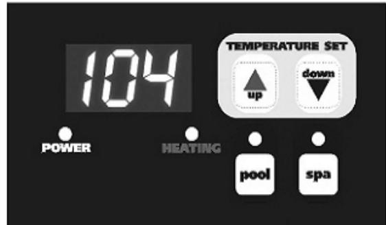
To enter *standby* mode: If *pool* mode is active (indicated by the green led over the *pool* button), press the *pool* button once. Rolling dots should appear on the display. If *spa* mode is active (indicated by the green led over the *spa* button), press the *spa* button once. Rolling dots should appear on the display.
