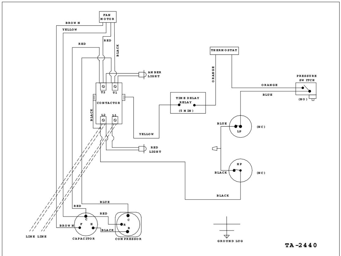
This wiring diagram is for use with all units that have **mechanical single thermostats**.
