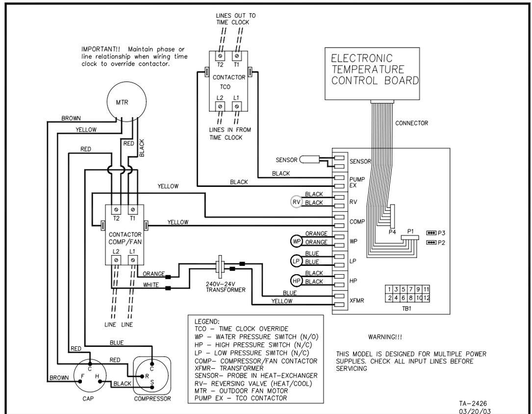
This wiring diagram is for use with all units that have *mechanical dual thermostats*.
