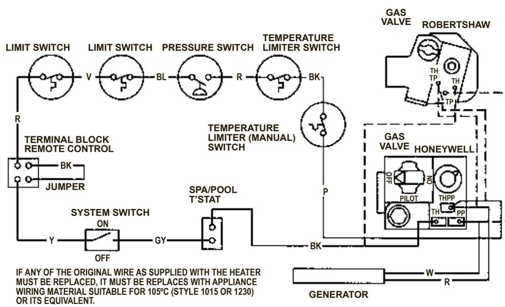
**Figure 30: Wiring Diagram - Millivolt**
