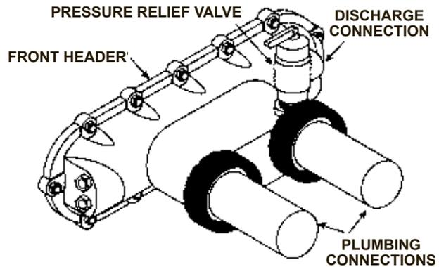
Figure 29: Pressure Relief Valve
