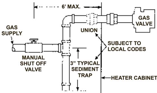
Figure 21: Sediment Trap
