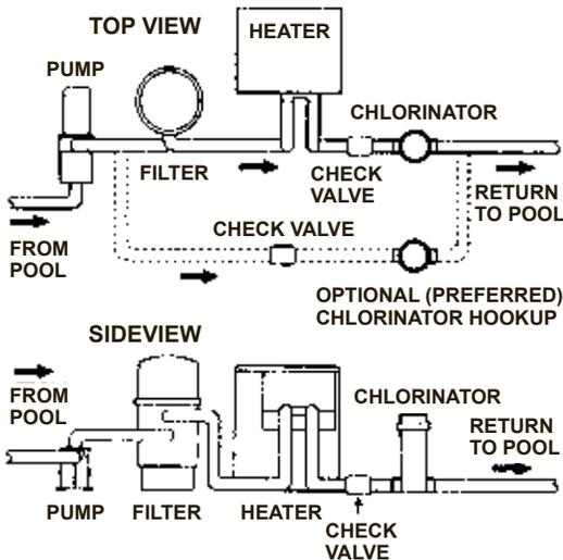
Figure 28: Automatic Chlorinator
