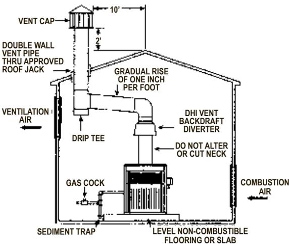
**Figure 17: Indoor Installation**
