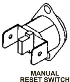
Figure 52: Limiter Switches
