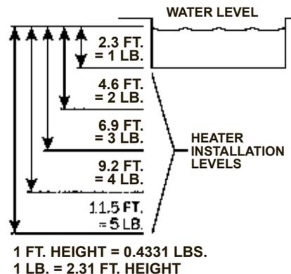
Figure 37: Heater Installation Below Pool
