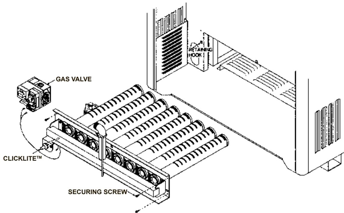
Figure 47: Burner Removal
