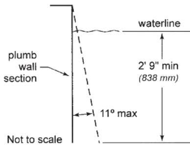
**Figure 2 Typical pool design configurations**
