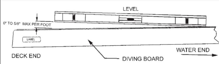
The top surface of the diving board from the deck end to the tip end shall be level or have an upward slope of 5/8” per foot maximum. Elevation difference shall not exceed 3-3/4” (6’ Board) or 5” (8’ Board) or 6-1/4” (10’ Board) from the deck end to the tip of the board. There shall be no downward slope towards the water. The slope shall be measured using a level as shown in the graphic to the left.
