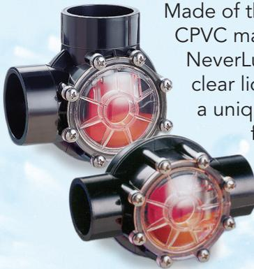
Made of the same tough CPVC material as the Jandy NeverLube® valve. It features a clear lid for easy inspection and a unique swing/spring design for both return and intake water. Available in straight or 90° models, 2" by 2½" or 2" by 1½" sizes.
