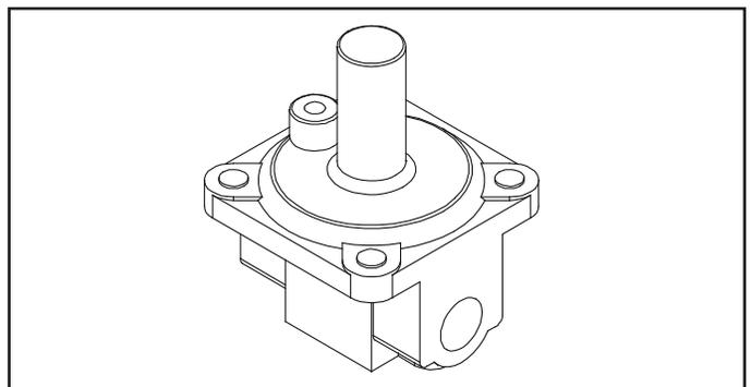
Figure 23. Step-down gas pressure regulator.
