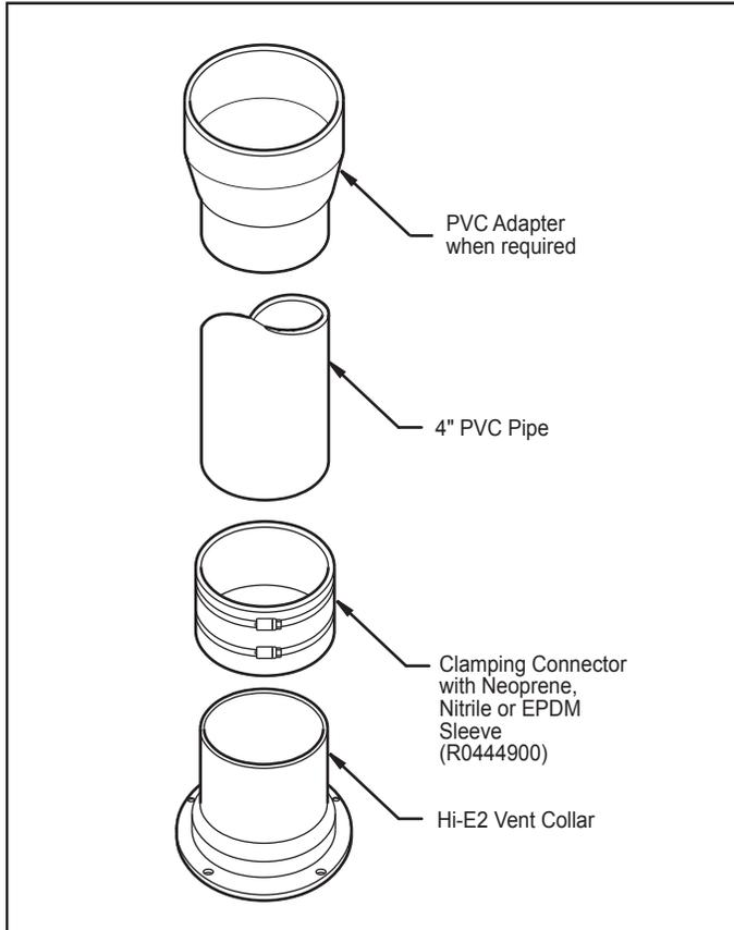
**Figure 7. Indoor vent connection, Hi-E2 pool heater.**
