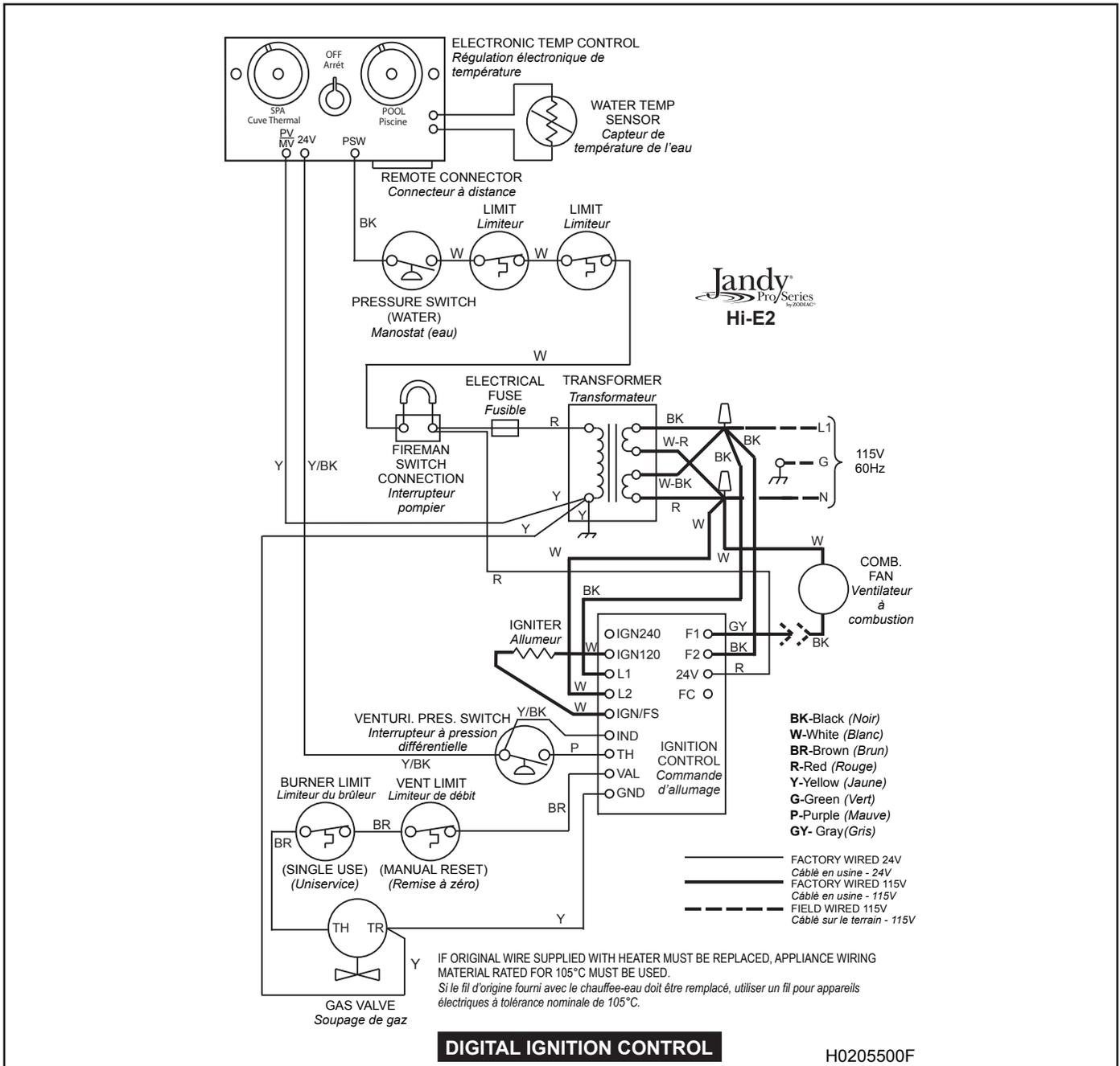
Figure 15. Wiring diagram, Hi-E2 pool heater.
