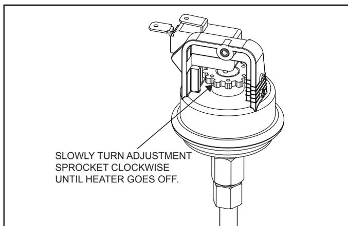
Figure 24. Adjustment of pressure switch.
