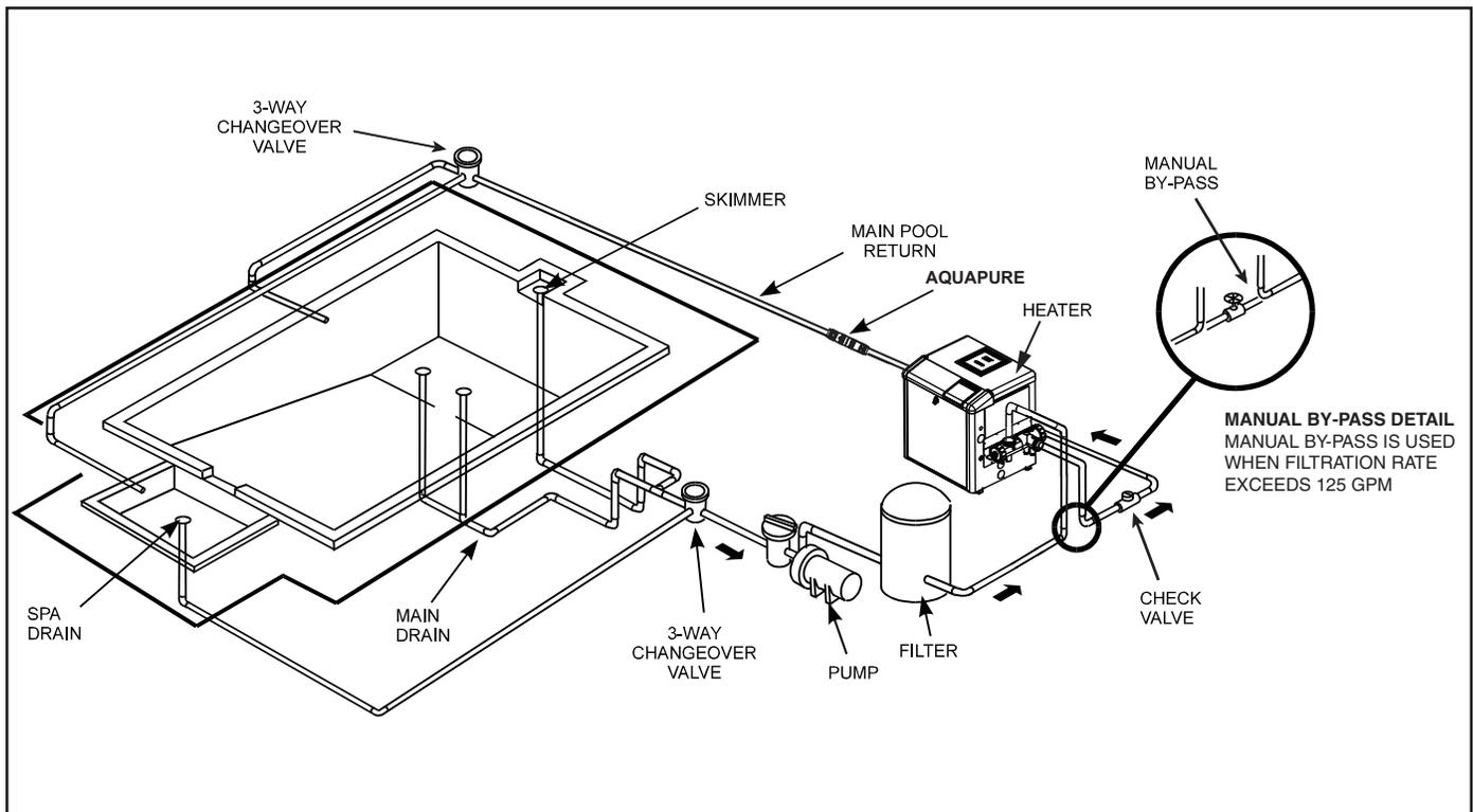
**Figure 20. Typical water piping.**
