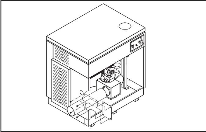
Figure 5. Connection of combustion air pipe to heater.
