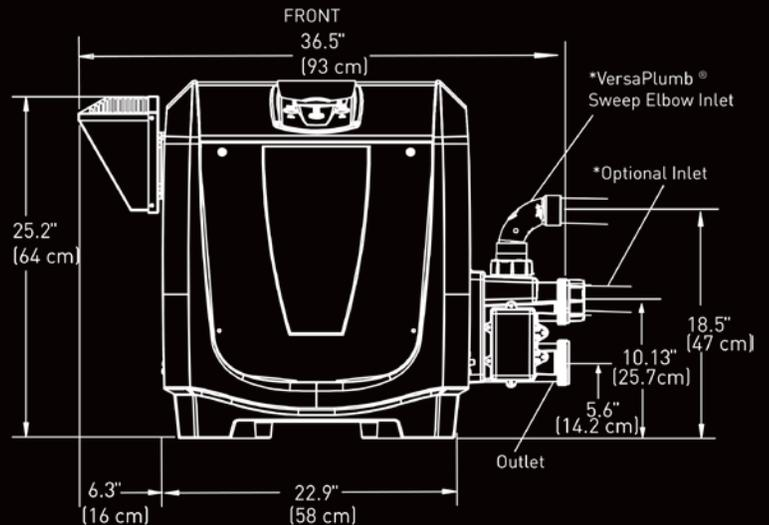
NOTE: Dimensions are identical on all heater models
