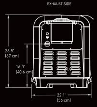
NOTE: Dimensions are identical on all heater models
