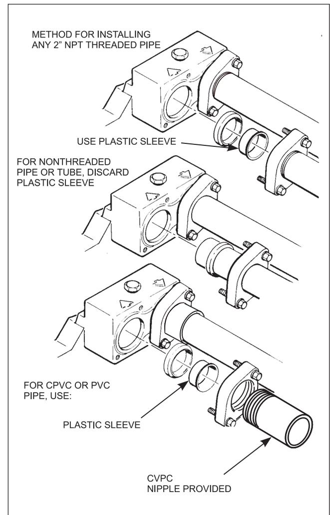
Figure 13. Piping installation
