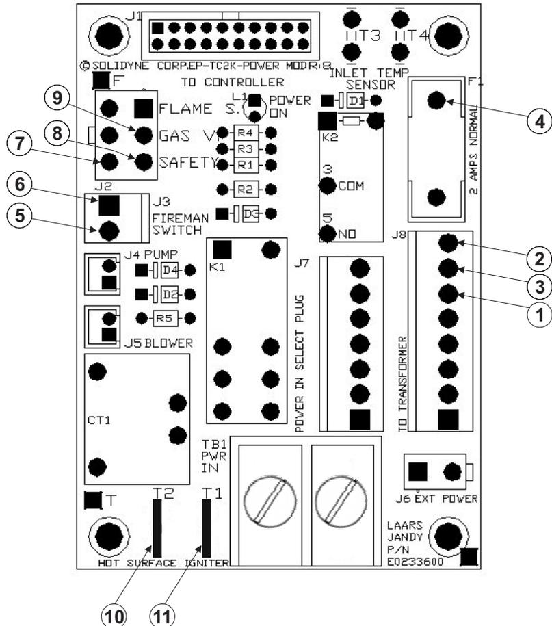
Figure 27. Power and Control Circuit Test Points
