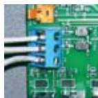
Figure 1. Remote Pool-Off- Spa Connection (3-Wire Connection)
