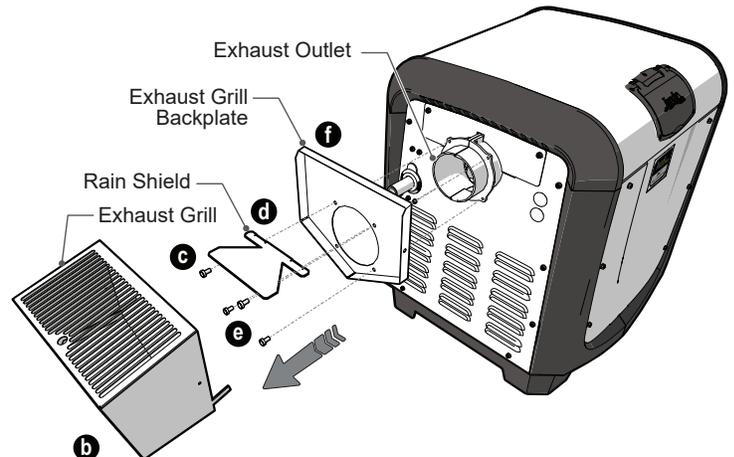
When the installation requires horizontal venting in excess of what is allowed for Category I installations or calls for horizontal discharge, the JXi may be installed with a Category III venting system.
