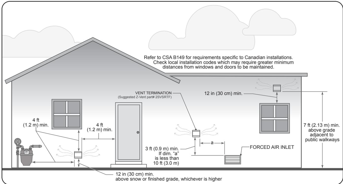
**Figure 7. Side Wall Vent Termination**
