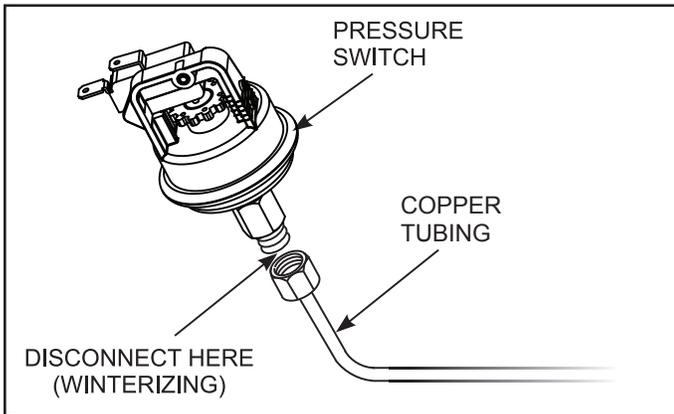
**Figure 22. Water Pressure Switch Copper Tubing (Siphon Loop)**
