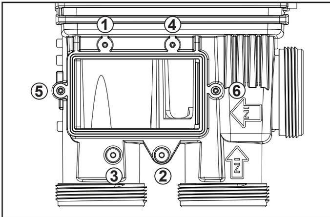
Figure 24. Header Bypass Reassembly Torque Pattern
