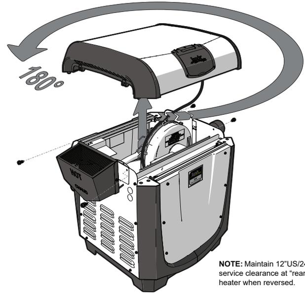
**NOTE:** Maintain 12" US/24" CAN service clearance at "rear" of heater when reversed.
