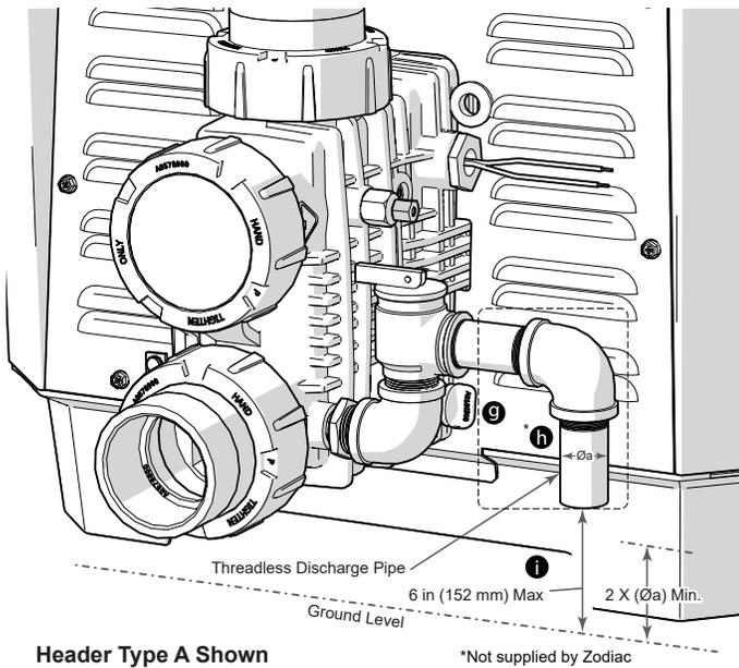
**h** Install a discharge pipe from the pressure relief valve discharge opening to a safe area. This is a precaution to prevent the possibility of personal injury or property damage in the event scalding water is discharged from the pressure relief valve.
