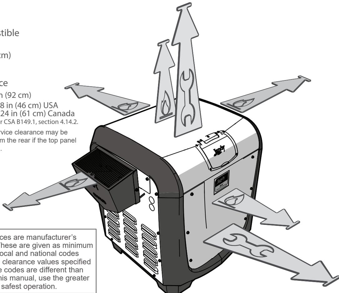
**NOTE:** Clearances are manufacturer's tested values. These are given as minimum values. Where local and national codes apply, and if the clearance values specified in the applicable codes are different than those listed in this manual, use the greater value to ensure safest operation.
