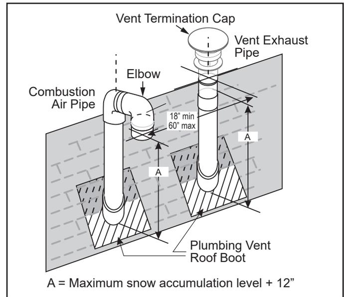
**Figure 6. Vent and combustion air terminals at roof.**
