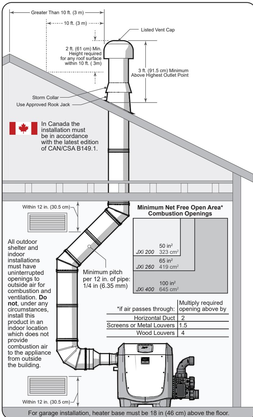
As outlined in the latest edition of ANSI® standard Z223.1 (NFPA® 54), the heater location must be properly vented to provide sufficient air supply for proper combustion.
