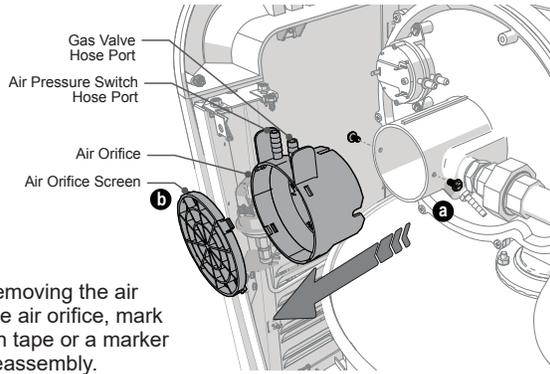
**TIP:** When removing the air hoses from the air orifice, mark the hoses with tape or a marker to help with reassembly.
