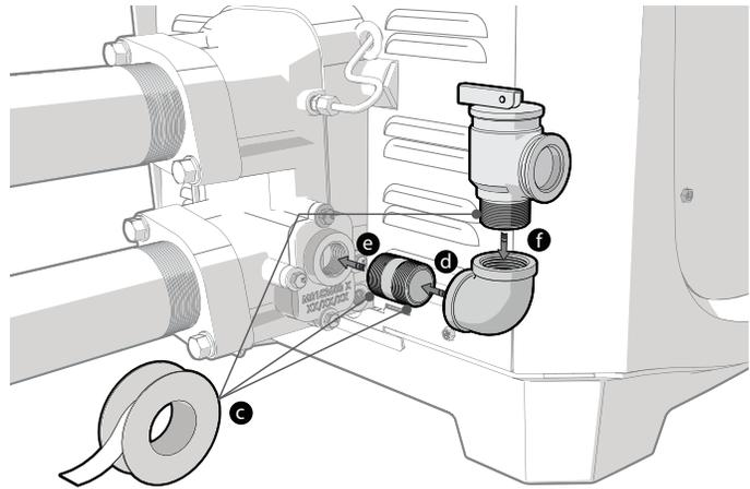
**f** Install the pressure relief valve. Make sure to get a snug fit. Do not overtighten.
