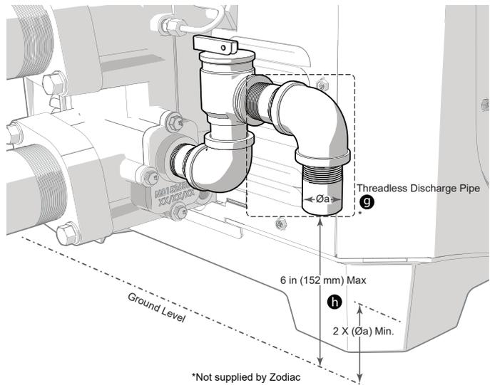
To ensure the continued proper operation of the pressure relief valve, the valve should be tested once a year. To test, lift the lever with the circulation system running to ensure that water will pass through. When the lever is down, there should be no leaks from the outlet.
