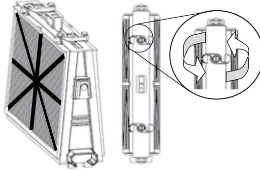
Reinstall the filters according to the diagram
