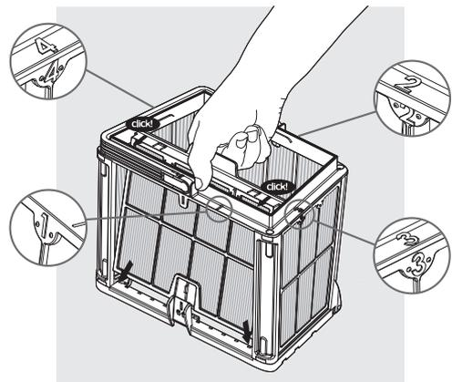
**8.2.5** Assemble the filter panels according to the following order: Panel 4 → 3 → 2 → 1.
