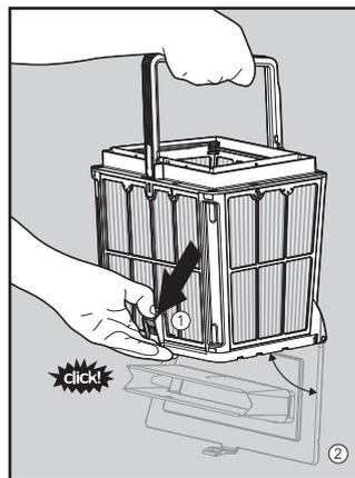
8.1.4 The debris can then be removed.
