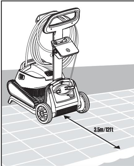
**5.1.1** Position the power supply so that it is approximately in the middle of the long side of the pool at a distance of 3.5m/12ft.
