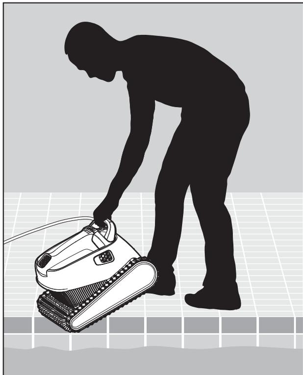
**5.2.1** Place the Pool Cleaner into the pool. Release the Pool Cleaner and let it sink to the floor of the pool. Make sure that the blue cable is free of any obstructions.
