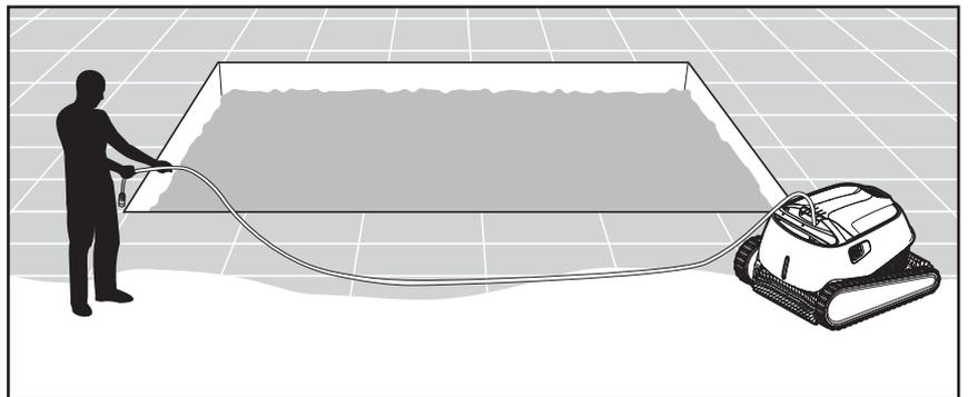
**5.1.2** Unwind the blue cable and stretch it out completely so that it has no kinks.
