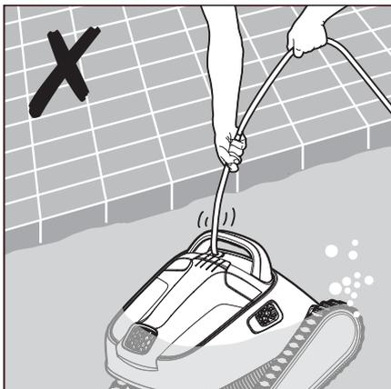
5.4.2 Using the blue cable, bring the Pool Cleaner to the pool edge. Use the handle to remove the Pool Cleaner from the pool.
