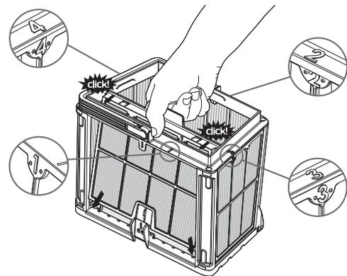
**8.2.5** Reassemble the filter panels in the order 4 → 3 → 2 → 1.
