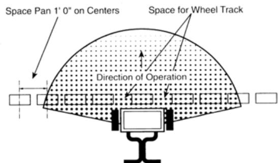
Once the pattern is uniform, the effective pattern width can be determined. The effective pattern width is the distance out from the spreader to a point where the amount of material is  $\frac{1}{2}$  the average amount in the center pans. This distance is multiplied by 2 to achieve the total effective pattern width.
