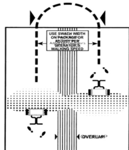
6) Push spreader at normal walking speed 2 ½ mph (18ft in 5 seconds). Apply header strips around area to be treated. Space trips across the area as shown. Keep material off flower bed, sidewalks, etc.
