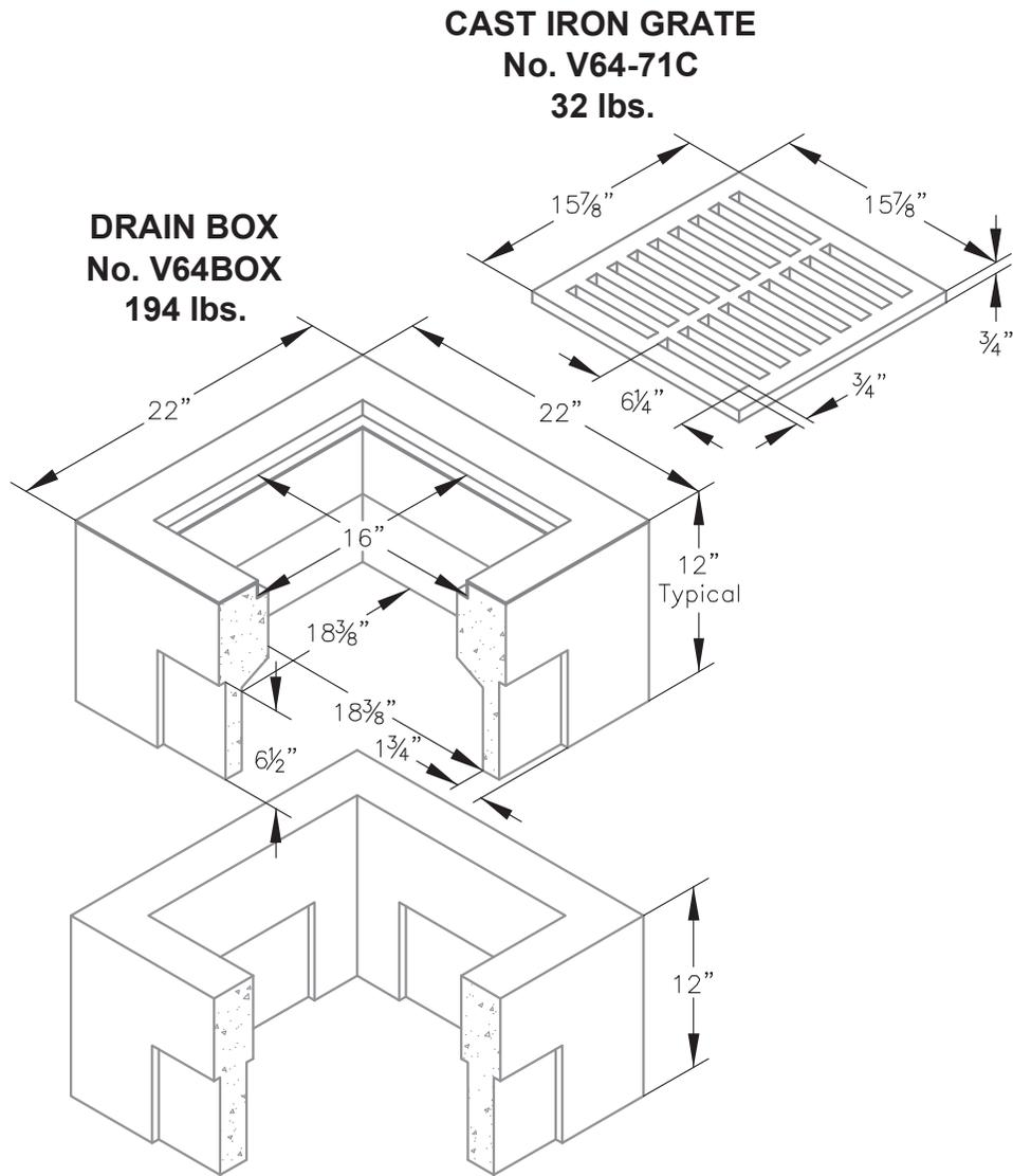
This concrete drain box has a cast in galvanized frame and is specifically engineered for drainage in medium areas such as parking lots, school grounds, walkways, ect. Its design permits final grading material to "lock in" and finish clean. Knock-outs accommodate up to 8" O.D. pipe. Approximate dimensions and weight shown. Also available in bolt down.
