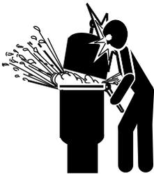
THIS FILTER OPERATES UNDER HIGH PRESSURE. WHEN ANY PART OF THE CIRCULATING SYSTEM (e.g. LOCK RING, PUMP, FILTER VALVES, ETC.) IS SERVICED, AIR CAN ENTER THE SYSTEM AND BECOME PRESSURIZED. PRESSURIZED AIR CAN CAUSE THE LID TO SERPARATE WHICH CAN RESULT IN SEVERE INJURY, DEATH, OR PROPERTY DAMAGE. TO AVOID THIS POTENTIAL HAZARD, FOLLOW THESE INSTRUCTIONS.
