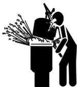
If the filter lock ring is damaged, replace it immediately. This filter operates under high pressure. Replace locking ring if damaged or worn. Failure to replace locking ring can result in the lid separating from the filter, which can cause severe injury or death.
