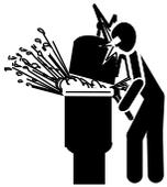
THIS FILTER OPERATES UNDER HIGH PRESSURE. WHEN ANY PART OF THE CIRCULATING SYSTEM (e.g. LOCK RING, PUMP, FILTER, VALVES, ETC.) IS SERVICED, AIR CAN ENTER THE SYSTEM AND BECOME PRESSURIZED. PRESSURIZED AIR CAN CAUSE THE LID TO SEPARATE WHICH CAN RESULT IN SEVERE INJURY, DEATH, OR PROPERTY DAMAGE.
