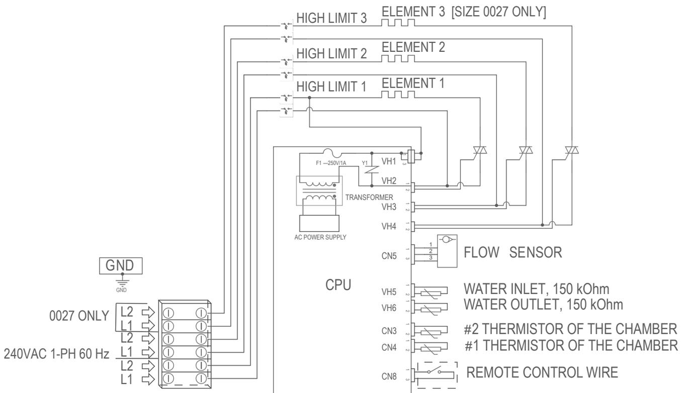
Figure 7. Wiring Diagram for Models ELS 0018 and 0027
