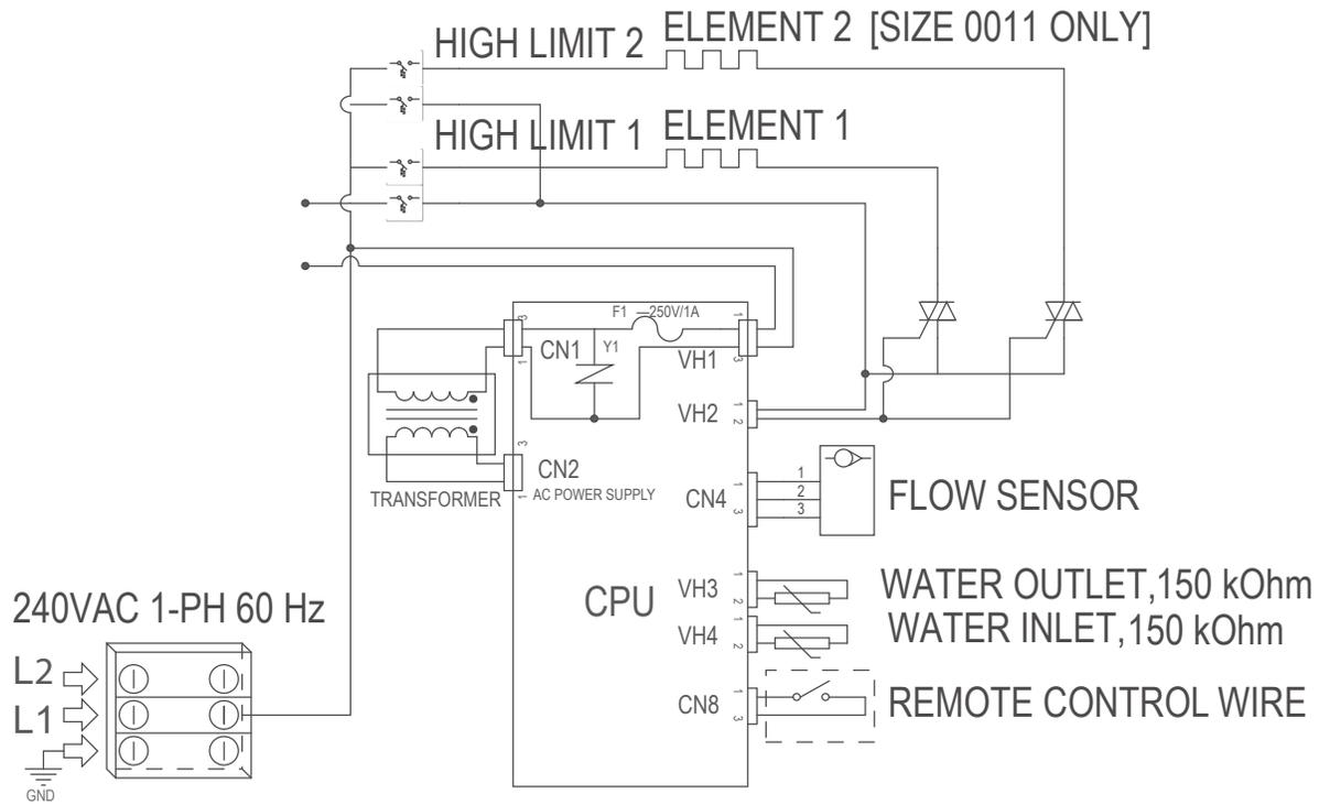
Figure 6. Wiring Diagram for Models ELS 0005 and 0011
