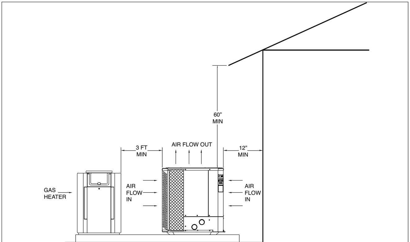
**Fig. 1: Installation Clearances**
