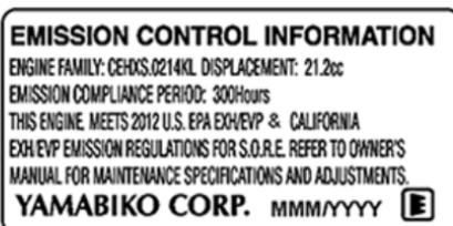
The 50 or 300 hour emission compliance period is the time span selected by the manufacturer certifying the engine emissions output meets applicable emissions regulations, provided that approved maintenance procedures are followed as listed in the Maintenance Section of this manual.
