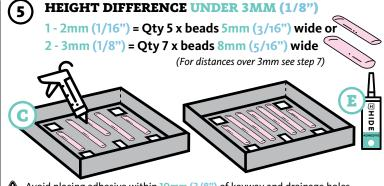
Avoid placing adhesive within 10mm (3/8") of keyway and drainage holes. Ensure the adhesive supports each corner of the inlay material. Ensure all bonding materials are fully dry.
