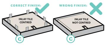
Make sure the glue has stiffened and remains flush with the inlay cover. Use tile spacers to center the infill.
