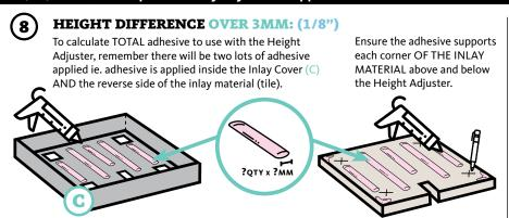
Place Height Adjuster on inlay (tile), then flip Inlay Cover (C) over and press down onto Height Adjuster (B):
