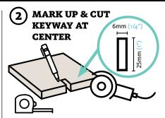
Ensure keyway is positioned on the tile edge which will be closest to the pool. Check that the key fits the keyway before gluing.
