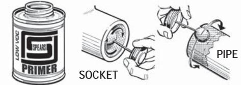
2. Apply primer to pipe in the same manner, extending application area to slightly more than the insertion depth into the valve socket.
