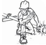
**WARNING:** SINGLE ENTRY BALL VALVES DO NOT USE A BLOCKED SEAL CARRIER ON THE UNION END AND CARRIER MAY BLOW OUT UNDER PRESSURE. DO NOT REMOVE OR LOOSEN THE UNION NUT WHILE THE VALVE IS UNDER PRESSURE.
