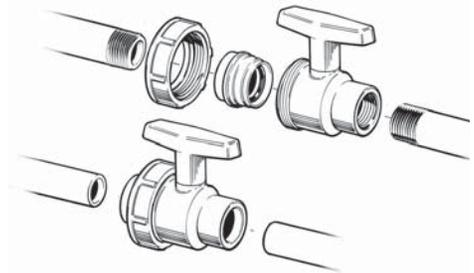
Valves are equipped with a union nut for valve seat adjustment and internal component servicing or replacement. Valves are factory pre-adjusted and removal of the single union nut and end connector is not required for general installation. However, these may be removed if needed for specific installation needs or convenience.
