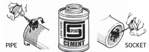
**VALVE INSTALLATION CAUTION: TAKE EXTRA CARE THAT NO PRIMER OR SOLVENT CEMENT IS ALLOWED TO CONTACT THE BALL OR OTHER INTERNAL VALVE COMPONENTS.**
