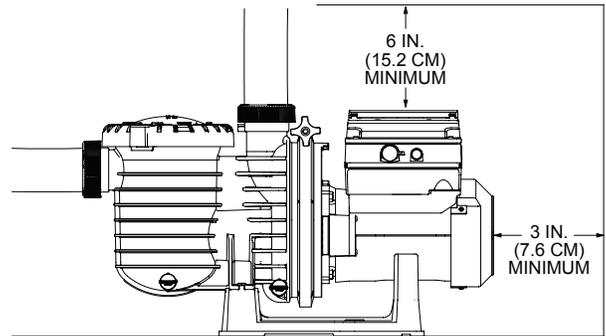
Figure 1: Pump Rear and Overhead Clearance
