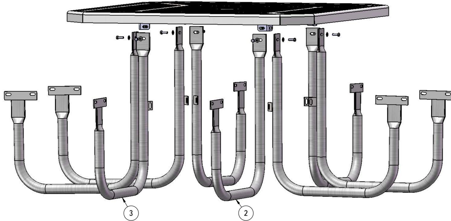
Attach the 358 Legs to the Extension Tabs using specified hardware.
