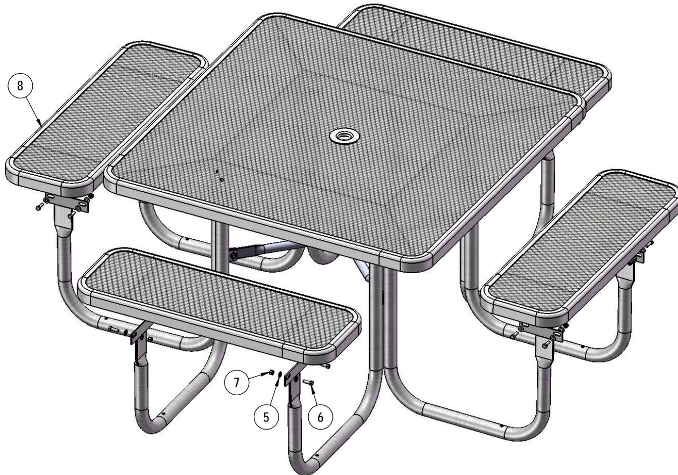
Attach the 3' Seats to the 358 Legs using specified hardware.
