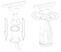
NOTE: You should not need to apply excessive force in order to close the latch. If you have trouble, make sure the filter bag is not between the seal and the nose cap or funnel and there are no other obstructions such as dirt or sand.
